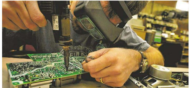
Chad Phillips, owner of For Your Listening Pleasure, removes the solder so he can take out the voltage regulator on a 2006 Toshiba flat-screen TV.
